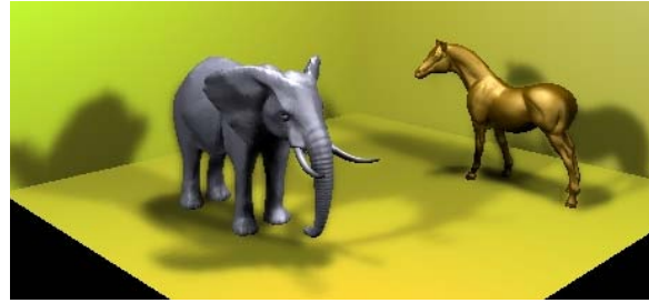
Figure 8: Close-up of a more complex scene using 3 point lights and 20 shadow ray samples rendered in 3268 ms using the visibility fields method. The BVH GPU method for sharp shadows takes 48047 ms.
