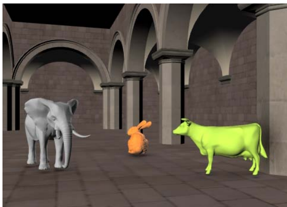
Figure 6: A scene of the Sponza Atrium with a bunny (38889 tris), a cow (92864 tris) and an elephant (157160 tris) rendered in three passes (one per object) with the visibility fields algorithm using 4226x64x64 maps and rendering in 2.5 frames per second.
