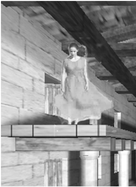
Figure 3: A Video source (girl) is superimposed as a billboard in the scene. The partial silhouette haloing is a result of the chroma-keyed transparent cloth and hair.
