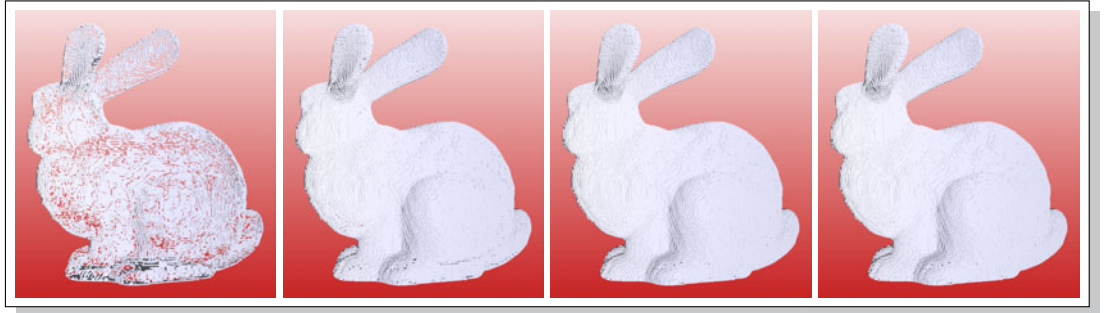
Figure 6.9: Comparison of the voxelization using the pixel shader clipping method at 256^3 volume resolution with 3, 6, 9 and 12 geometry shader vertices output. The number of voxels produced are 52382, 87690 and 89696 (complete voxelization) for 3, 6, 9 and above geometry shader output vertices, respectively.
