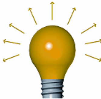
Figure 2.3: The radiant power \Phi of a light source is given by its total emitted radiation.
