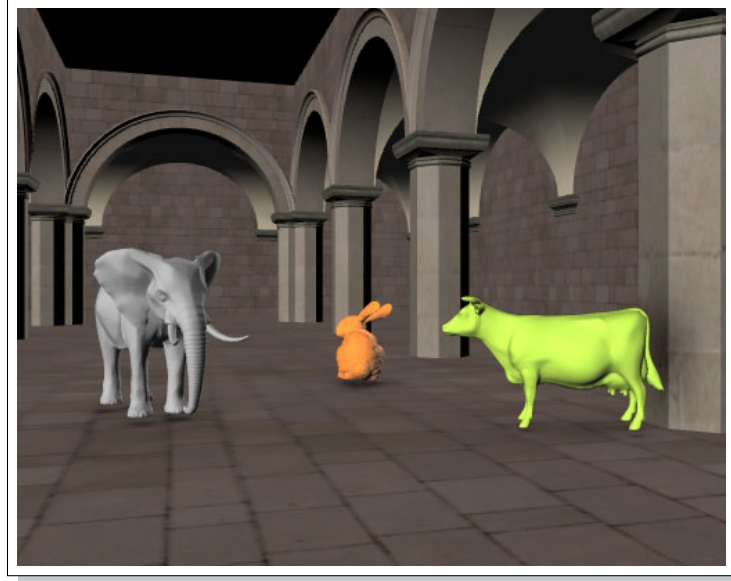
Figure 4.15: A scene of the Sponza Atrium with a bunny (38889 tris), a cow (92864 tris) and an elephant (157160 tris) rendered in three passes (one per object) with the visibility fields algorithm using 4226x64x64 maps and rendering in 2.5 frames per second.
