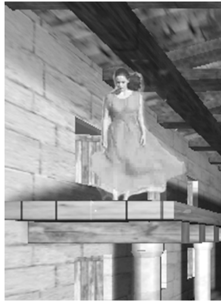
Figure 2: A Video source (girl) is superimposed as a billboard in the scene. The partial silhouette haloing is a result of the chroma-keyed transparent cloth and hair.
